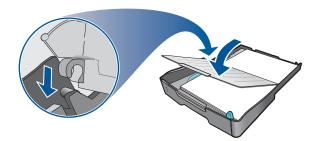
6 Insert the tray back into the printer.
